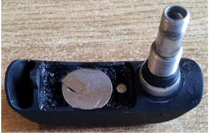
Using the knife blade, tease the edges of the +ve terminal plate up off the surface of the battery on each side of the two spot welds.
